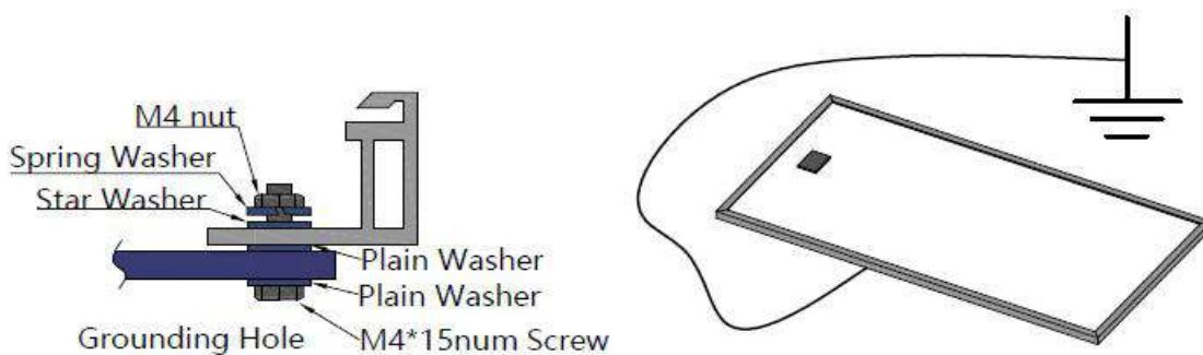
Figure 8: Ground installation of PV modules
